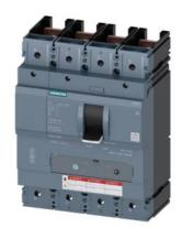
CIRCUIT BREAKER 3VA5 UL FRAME 400 BREAKING CAPACITY CLASS C 100kA @ 480 V 4POLE, LINE PROTECTION TM240, ATAM, In=400A OVERLOAD PROTECTION IR=280A ...400A SHORT CIRCUIT PROTECTION II=5...10 X IN NEUTRAL UNPROTECTED W/O CONNECTION
