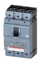
CIRCUIT BREAKER 3VA5 UL FRAME 400 BREAKING CAPACITY CLASS C 100kA @ 480 V 3POLE, LINE PROTECTION TM240, ATAM, In=400A OVERLOAD PROTECTION Ir=280A ...400A SHORT CIRCUIT PROTECTION Ii=5...10 x In ALLUG LINE AND LOAD SIDE
