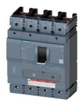
CIRCUIT BREAKER 3VA5 UL FRAME 400 BREAKING CAPACITY CLASS C 100kA @ 480 V 4POLE, LINE PROTECTION TM230, FTAM, In=400A OVERLOAD PROTECTION IR=400A FIXED SHORT CIRCUIT PROTECTION II=5...10 X IN NEUTRAL UNPROTECTED W/O CONNECTION
