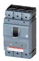
CIRCUIT BREAKER 3VA5 UL FRAME 400 BREAKING CAPACITY CLASS C 100kA @ 480 V 3POLE, LINE PROTECTION TM230, FTAM, In=400A OVERLOAD PROTECTION Ir=400A FIXED SHORT CIRCUIT PROTECTION Ii=5...10 x In ALLUG LINE AND LOAD SIDE
