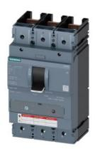
CIRCUIT BREAKER 3VA5 UL Frame 400 BREAKING CAPACITY CLASS H 65kA @ 480 V 3POLE, LINE PROTECTION TM240, ATAM, In=400A OVERLOAD PROTECTION IR=280A ...400A SHORT CIRCUIT PROTECTION Ii=5...10 x In W/O CONNECTION
