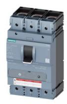
CIRCUIT BREAKER 3VA5 UL Frame 400 BREAKING CAPACITY CLASS H 65kA @ 480 V 3POLE, LINE PROTECTION TM230, FTAM, In=400A OVERLOAD PROTECTION Ir=400A FIXED SHORT CIRCUIT PROTECTION Ii=5...10 x In ALLUG LINE AND LOAD SIDE
