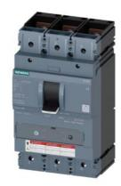
CIRCUIT BREAKER 3VA5 UL Frame 400 BREAKING CAPACITY CLASS H 65kA @ 480 V 3POLE, LINE PROTECTION TM230, FTAM, In=400A OVERLOAD PROTECTION Ir=400A FIXED SHORT CIRCUIT PROTECTION Ii=5...10 x In NUT KEEPER KIT LINE AND LOAD S.
