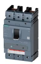
CIRCUIT BREAKER 3VA5 UL Frame 400 BREAKING CAPACITY CLASS M 35kA @ 480 V 2POLE, LINE PROTECTION TM230, FTAM, In=400A OVERLOAD PROTECTION IR=400A FIXED SHORT CIRCUIT PROTECTION Ii=5...10 x In W/O CONNECTION
