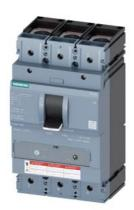
CIRCUIT BREAKER 3VA5 UL Frame 400 BREAKING CAPACITY CLASS M 35kA @ 480 V 3POLE, LINE PROTECTION TM230, FTAM, In=400A OVERLOAD PROTECTION Ir=400A FIXED SHORT CIRCUIT PROTECTION Ii=5...10 x In ALLUG LINE AND LOAD SIDE
