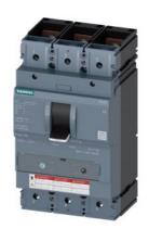
CIRCUIT BREAKER 3VA5 UL Frame 400 BREAKING CAPACITY CLASS M 35kA @ 480 V 3POLE, LINE PROTECTION TM230, FTAM, In=400A OVERLOAD PROTECTION Ir=400A FIXED SHORT CIRCUIT PROTECTION Ii=5...10 x In UL489 SB (NAVAL), 50 DEG CEL. NUT KEEPER KIT LINE AND LOAD S.
