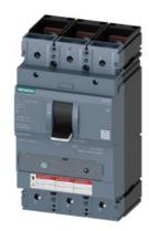
CIRCUIT BREAKER 3VA5 UL Frame 400 BREAKING CAPACITY CLASS M 35kA @ 480 V 3POLE, LINE PROTECTION TM230, FTAM, In=400A OVERLOAD PROTECTION Ir=400A FIXED SHORT CIRCUIT PROTECTION Ii=5...10 x In NUT KEEPER KIT LINE AND LOAD S.
