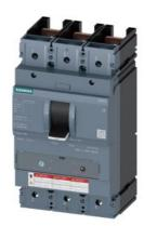
CIRCUIT BREAKER 3VA5 UL Frame 400 BREAKING CAPACITY CLASS M 35kA @ 480 V 3POLE, LINE PROTECTION TM230, FTAM, In=400A OVERLOAD PROTECTION IR=400A FIXED SHORT CIRCUIT PROTECTION Ii=5...10 x In W/O CONNECTION
