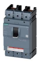
MOLDED CASE SWITCH 3VA5 UL FRAME 400 MAX SHORT CIRCUIT CURR. RATING 100kA @ 480 V 2POLE, LINE PROTECTION MCS110, In=400A WITHOUT OVERLOAD PROTECTION SELF PROTECTION Ii=15 x In W/O CONNECTION
