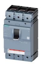
MOLDED CASE SWITCH 3VA5 UL FRAME 400 MAX SHORT CIRCUIT CURR. RATING 100kA @ 480 V 3POLE, LINE PROTECTION MCS110, In=400A WITHOUT OVERLOAD PROTECTION SELF PROTECTION Ii=10 x In ALLUG LINE AND LOAD SIDE
