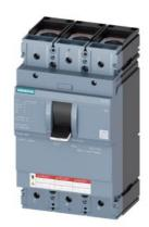
MOLDED CASE SWITCH 3VA5 UL FRAME 400 MAX SHORT CIRCUIT CURR. RATING 65kA @ 480 V 3POLE, LINE PROTECTION MCS110, In=400A WITHOUT OVERLOAD PROTECTION SELF PROTECTION Ii=10 x In ALLUG LINE AND LOAD SIDE
