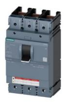
MOLDED CASE SWITCH 3VA5 UL FRAME 400 MAX SHORT CIRCUIT CURR. RATING 65kA @ 480 V 3POLE, LINE PROTECTION MCS110, In=400A WITHOUT OVERLOAD PROTECTION SELF PROTECTION Ii=15 x In W/O CONNECTION
