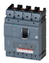
CIRCUIT BREAKER 3VA5 UL Frame 400 BREAKING CAPACITY CLASS H 65kA @ 480 V 4POLE, LINE PROTECTION TM230, FTAM, In=350A OVERLOAD PROTECTION IR=350A FIXED SHORT CIRCUIT PROTECTION Ii=5...10 x In NEUTRAL UNPROTECTED W/O CONNECTION
