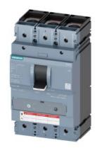
CIRCUIT BREAKER 3VA5 UL FRAME 400 BREAKING CAPACITY CLASS C 100kA @ 480 V 3POLE, LINE PROTECTION TM230, FTAM, In=300A OVERLOAD PROTECTION Ir=300A FIXED SHORT CIRCUIT PROTECTION Ii=5...10 x In UL489 SB (NAVAL), 50 DEG CEL. ALLUG LINE AND LOAD SIDE
