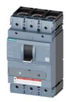
CIRCUIT BREAKER 3VA5 UL FRAME 400 BREAKING CAPACITY CLASS C 100kA @ 480 V 3POLE, LINE PROTECTION TM230, FTAM, In=300A OVERLOAD PROTECTION Ir=300A FIXED SHORT CIRCUIT PROTECTION Ii=5...10 x In ALLUG LINE AND LOAD SIDE
