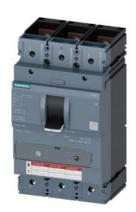
CIRCUIT BREAKER 3VA5 UL FRAME 400 BREAKING CAPACITY CLASS C 100kA @ 480 V 3POLE, LINE PROTECTION TM230, FTAM, In=300A OVERLOAD PROTECTION Ir=300A FIXED SHORT CIRCUIT PROTECTION Ii=5...10 x In UL489 SB (NAVAL), 50 DEG CEL. NUT KEEPER KIT LINE AND LOAD S.
