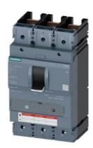
CIRCUIT BREAKER 3VA5 UL FRAME 400 BREAKING CAPACITY CLASS C 100kA @ 480 V 3POLE, LINE PROTECTION TM230, FTAM, In=300A OVERLOAD PROTECTION IR=300A FIXED SHORT CIRCUIT PROTECTION II=5...10 X IN UL489 SB (NAVAL), 50 DEG CEL. W/O CONNECTION
