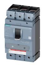
CIRCUIT BREAKER 3VA5 UL Frame 400 BREAKING CAPACITY CLASS M 35kA @ 480 V 3POLE, LINE PROTECTION TM230, FTAM, In=300A OVERLOAD PROTECTION Ir=300A FIXED SHORT CIRCUIT PROTECTION Ii=5...10 x In UL489 SB (NAVAL), 50 DEG CEL. ALLUG LINE AND LOAD SIDE
