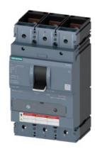
CIRCUIT BREAKER 3VA5 UL FRAME 400 BREAKING CAPACITY CLASS C 100kA @ 480 V 3POLE, LINE PROTECTION TM230, FTAM, In=250A OVERLOAD PROTECTION Ir=250A FIXED SHORT CIRCUIT PROTECTION Ii=5...10 x In NUT KEEPER KIT LINE AND LOAD S.
