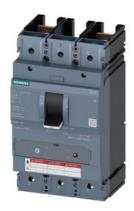
CIRCUIT BREAKER 3VA5 UL Frame 400 BREAKING CAPACITY CLASS M 35kA @ 480 V 2POLE, LINE PROTECTION TM230, FTAM, In=250A OVERLOAD PROTECTION IR=250A FIXED SHORT CIRCUIT PROTECTION Ii=5...10 x In W/O CONNECTION
