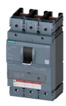
CIRCUIT BREAKER 3VA5 UL Frame 400 3POLE,MOTOR STARTER PROTECTION TM120M, AM, In=250A WITHOUT OVERLOAD PROTECTION SHORT CIRCUIT PROTECTION Ii=3...6 x In W/O CONNECTION
