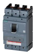
CIRCUIT BREAKER 3VA5 UL Frame 400 3POLE,MOTOR STARTER PROTECTION TM120M, AM, In=250A WITHOUT OVERLOAD PROTECTION SHORT CIRCUIT PROTECTION Ii=6...12 x In W/O CONNECTION
