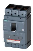
CIRCUIT BREAKER 3VA5 UL FRAME 400 BREAKING CAPACITY CLASS C 100kA @ 480 V 3POLE, LINE PROTECTION TM240, ATAM, In=225A OVERLOAD PROTECTION Ir=157,5A ...225A SHORT CIRCUIT PROTECTION Ii=5...10 x In NUT KEEPER KIT LINE AND LOAD S.
