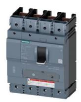
CIRCUIT BREAKER 3VA5 UL FRAME 400 BREAKING CAPACITY CLASS C 100kA @ 480 V 4POLE, LINE PROTECTION TM230, FTAM, In=225A OVERLOAD PROTECTION IR=225A FIXED SHORT CIRCUIT PROTECTION II=5...10 X IN NEUTRAL UNPROTECTED W/O CONNECTION
