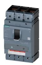
CIRCUIT BREAKER 3VA5 UL FRAME 400 BREAKING CAPACITY CLASS C 100kA @ 480 V 3POLE, LINE PROTECTION TM230, FTAM, In=225A OVERLOAD PROTECTION Ir=225A FIXED SHORT CIRCUIT PROTECTION Ii=5...10 x In UL489 SB (NAVAL), 50 DEG CEL. NUT KEEPER KIT LINE AND LOAD S.
