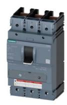
CIRCUIT BREAKER 3VA5 UL FRAME 400 BREAKING CAPACITY CLASS C 100kA @ 480 V 3POLE, LINE PROTECTION TM230, FTAM, In=225A OVERLOAD PROTECTION IR=225A FIXED SHORT CIRCUIT PROTECTION II=5...10 X IN UL489 SB (NAVAL), 50 DEG CEL. W/O CONNECTION
