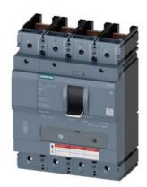
CIRCUIT BREAKER 3VA5 UL Frame 400 BREAKING CAPACITY CLASS H 65kA @ 480 V 4POLE, LINE PROTECTION TM230, FTAM, In=225A OVERLOAD PROTECTION IR=225A FIXED SHORT CIRCUIT PROTECTION Ii=5...10 x In NEUTRAL UNPROTECTED W/O CONNECTION
