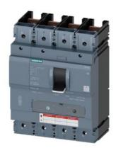
CIRCUIT BREAKER 3VA5 UL FRAME 400 BREAKING CAPACITY CLASS C 100kA @ 480 V 4POLE, LINE PROTECTION TM240, ATAM, In=200A OVERLOAD PROTECTION IR=140A ...200A SHORT CIRCUIT PROTECTION II=5...10 X IN NEUTRAL PROTECTION 100% W/O CONNECTION
