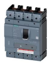
CIRCUIT BREAKER 3VA5 UL FRAME 400 BREAKING CAPACITY CLASS C 100kA @ 480 V 4POLE, LINE PROTECTION TM230, FTAM, In=200A OVERLOAD PROTECTION IR=200A FIXED SHORT CIRCUIT PROTECTION II=5...10 X IN NEUTRAL PROTECTION 100% W/O CONNECTION
