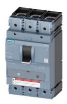
CIRCUIT BREAKER 3VA5 UL FRAME 400 BREAKING CAPACITY CLASS C 100kA @ 480 V 3POLE, LINE PROTECTION TM240, ATAM, In=200A OVERLOAD PROTECTION Ir=140A ...200A SHORT CIRCUIT PROTECTION Ii=5...10 x In ALLUG LINE AND LOAD SIDE
