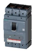
CIRCUIT BREAKER 3VA5 UL FRAME 400 BREAKING CAPACITY CLASS C 100kA @ 480 V 3POLE, LINE PROTECTION TM240, ATAM, In=200A OVERLOAD PROTECTION Ir=140A ...200A SHORT CIRCUIT PROTECTION Ii=5...10 x In NUT KEEPER KIT LINE AND LOAD S.
