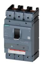
CIRCUIT BREAKER 3VA5 UL FRAME 400 BREAKING CAPACITY CLASS C 100kA @ 480 V 3POLE, LINE PROTECTION TM240, ATAM, In=200A OVERLOAD PROTECTION IR=140A ...200A SHORT CIRCUIT PROTECTION II=5...10 X IN W/O CONNECTION
