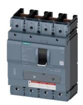
CIRCUIT BREAKER 3VA5 UL FRAME 400 BREAKING CAPACITY CLASS C 100kA @ 480 V 4POLE, LINE PROTECTION TM230, FTAM, In=200A OVERLOAD PROTECTION IR=200A FIXED SHORT CIRCUIT PROTECTION II=5...10 X IN NEUTRAL UNPROTECTED W/O CONNECTION
