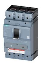
CIRCUIT BREAKER 3VA5 UL FRAME 400 BREAKING CAPACITY CLASS C 100kA @ 480 V 3POLE, LINE PROTECTION TM230, FTAM, In=200A OVERLOAD PROTECTION Ir=200A FIXED SHORT CIRCUIT PROTECTION Ii=5...10 x In UL489 SB (NAVAL), 50 DEG CEL. ALLUG LINE AND LOAD SIDE
