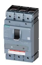
CIRCUIT BREAKER 3VA5 UL FRAME 400 BREAKING CAPACITY CLASS C 100kA a 480 V 3POLE, LINE PROTECTION TM230, FTAM, In=200A OVERLOAD PROTECTION Ir=200A FIXED SHORT CIRCUIT PROTECTION Ii=5...10 x In ALLUG LINE AND LOAD SIDE
