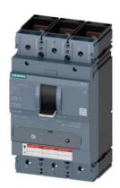
CIRCUIT BREAKER 3VA5 UL FRAME 400 BREAKING CAPACITY CLASS C 100kA @ 480 V 3POLE, LINE PROTECTION TM230, FTAM, In=200A OVERLOAD PROTECTION Ir=200A FIXED SHORT CIRCUIT PROTECTION Ii=5...10 x In UL489 SB (NAVAL), 50 DEG CEL. NUT KEEPER KIT LINE AND LOAD S.
