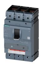
CIRCUIT BREAKER 3VA5 UL FRAME 400 BREAKING CAPACITY CLASS C 100kA @ 480 V 3POLE, LINE PROTECTION TM230, FTAM, In=200A OVERLOAD PROTECTION Ir=200A FIXED SHORT CIRCUIT PROTECTION Ii=5...10 x In NUT KEEPER KIT LINE AND LOAD S.
