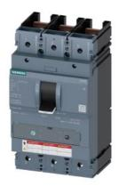
CIRCUIT BREAKER 3VA5 UL FRAME 400 BREAKING CAPACITY CLASS C 100kA @ 480 V 3POLE, LINE PROTECTION TM230, FTAM, In=200A OVERLOAD PROTECTION IR=200A FIXED SHORT CIRCUIT PROTECTION II=5...10 X IN UL489 SB (NAVAL), 50 DEG CEL. W/O CONNECTION
