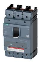
CIRCUIT BREAKER 3VA5 UL FRAME 400 BREAKING CAPACITY CLASS C 100kA @ 480 V 3POLE, LINE PROTECTION TM230, FTAM, In=200A OVERLOAD PROTECTION IR=200A FIXED SHORT CIRCUIT PROTECTION II=5...10 X IN W/O CONNECTION
