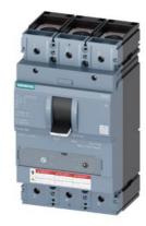
CIRCUIT BREAKER 3VA5 UL Frame 400 BREAKING CAPACITY CLASS H 65kA @ 480 V 3POLE, LINE PROTECTION TM230, FTAM, In=200A OVERLOAD PROTECTION Ir=200A FIXED SHORT CIRCUIT PROTECTION Ii=5...10 x In UL489 SB (NAVAL), 50 DEG CEL. ALLUG LINE AND LOAD SIDE
