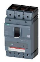
CIRCUIT BREAKER 3VA5 UL Frame 400 BREAKING CAPACITY CLASS H 65kA @ 480 V 3POLE, LINE PROTECTION TM230, FTAM, In=200A OVERLOAD PROTECTION Ir=200A FIXED SHORT CIRCUIT PROTECTION Ii=5...10 x In NUT KEEPER KIT LINE AND LOAD S.
