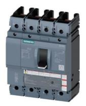
circuit breaker 3VA5 UL frame 250 breaking capacity class C 100kA @ 480V 4-pole, line protection TM210, FTFM, In=90A overload protection Ir=90A fixed short-circuit protection Ii=10 x In N conductor unprotected without connection
