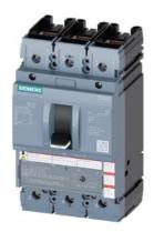
circuit breaker 3VA5 UL frame 250 breaking capacity class C 100kA @ 480 V 3-pole, line protection TM210, FTFM, In=90A overload protection Ir=90A fixed short-circuit protection Ii=10 x In cable connection on both sides
