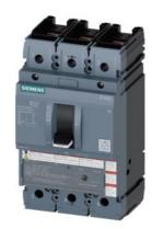
circuit breaker 3VA5 UL frame 250 breaking capacity class C 100kA @ 480 V 3-pole, line protection TM230, FTAM, In=90A overload protection Ir=90A fixed short-circuit protection Ii=5...10 x In UL489 SB (naval), 50 deg. cel. nut keeper kit on both sides
