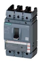
circuit breaker 3VA5 UL frame 250 breaking capacity class C 100kA @ 480V 3-pole, line protection TM230, FTAM, In=90A overload protection Ir=90A fixed short-circuit protection Ii=5...10 x In UL 489 SB (naval), 50 °C without connection
