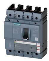
circuit breaker 3VA5 UL frame 250 breaking capacity class H 65kA @ 480V 4-pole, line protection TM230, FTAM, In=80A overload protection Ir=80A fixed short-circuit protection Ii=5...10 x In N conductor unprotected without connection
